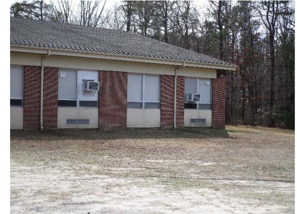
A rain garden can be installed at the northwestern corner of the school to capture, treat, and infiltrate rooftop runoff. A preliminary soil assessment suggests that the soils have suitable drainage characteristics for green infrastructure.
